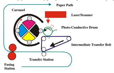
As you can tell in this printing scenario, it takes time to perform the mechanical activities of rotating the next toner cartridge into position and aligning the top of the color planes on to one another on a single intermediate transfer belt. You can also see why the HP Color LaserJet 4550 printer can print black (monochrome, one color plane images) at 16 pages per minute and color pages (four color plane images) at four pages per minute.
